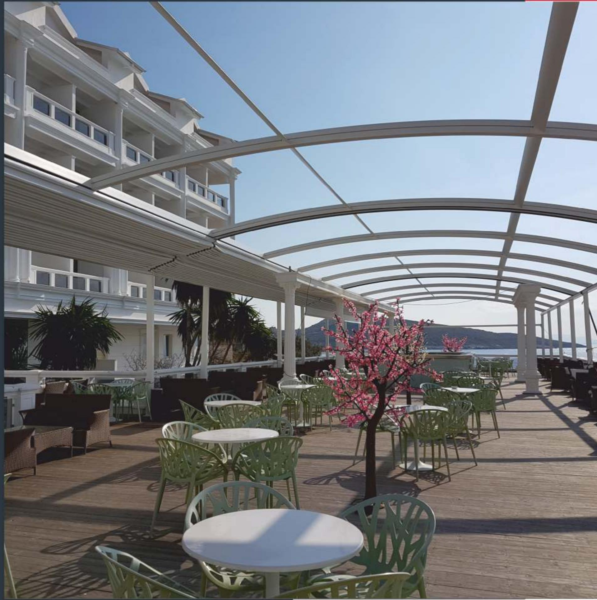
The VAULT Curved Rafter Profiles have been designed with smart side channels that allow an easy installation and side Waterguard Channels. Rafter profiles, including a timing belt of T10/33, are driven by patented six-wheel sliders with easy clip installation for fabric that allows a silent motion when the fabric is retracted. VAULT rafters are served with two different dimensions to provide a maximum range for extension values:
