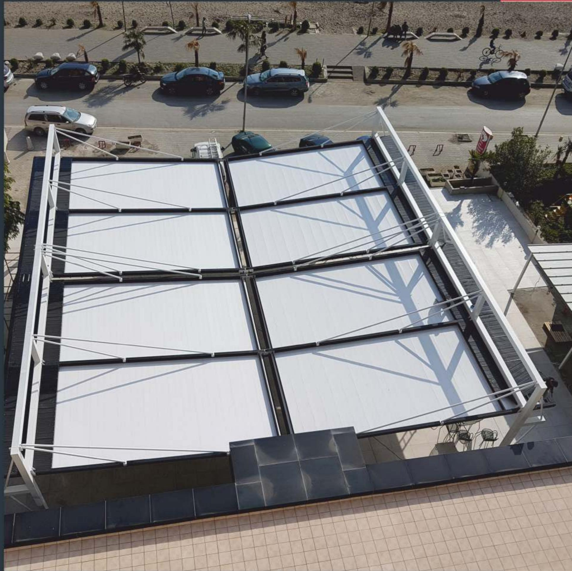
The FLAT CITY Rafter Profiles have been designed with smart side channels that allow easy installation and side Waterguard Channels. Rafter profiles, including a timing belt of T10/20, is driven by a patented six-wheel slider with an easy clip installation system that allows a silent motion when the fabric is retracted. FLAT CITY rafters are served with three different dimensions to provide a maximum range for extension values:
